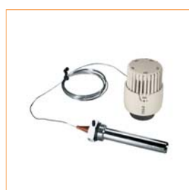
T 3011. Thermostatic head with integrated command and remote immersion probe. Adjustment range 20÷60 °C.
