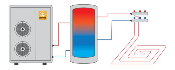
SmartHeat buffer tanks are designed to be used in hydronic heating systems with heat pumps, gas boilers and biomass/wood boilers. Using a buffer tank in hydronic systems assists efficiency operation by preventing the low-mass boiler from short cycling which can reduce the cause of failure in any type of hydronic heater.
