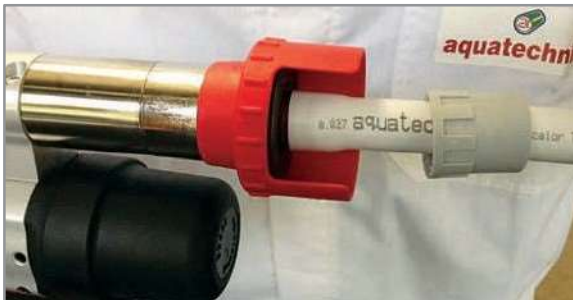
3 – Push the pipe up to the stop of the mechanical expander. Hold the trigger until the pipe is expanded (the pipe will be automatically released from the tool once the operation is completed).
